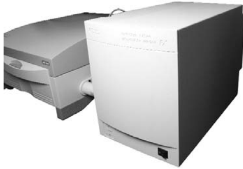
Fig. 4.7. PharosFX External Laser Module connected to the scanner
