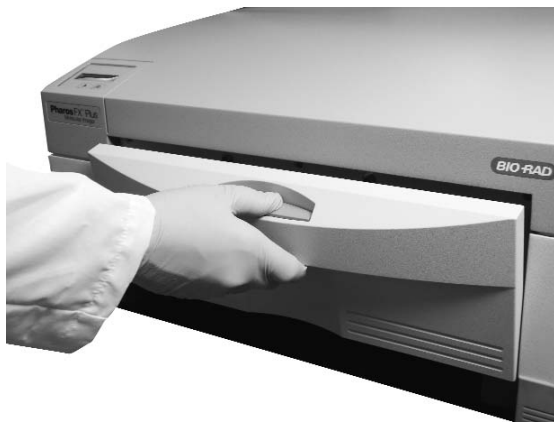
Fig. 4.2. Steps for inserting a fluorescent sample into the scanner.
