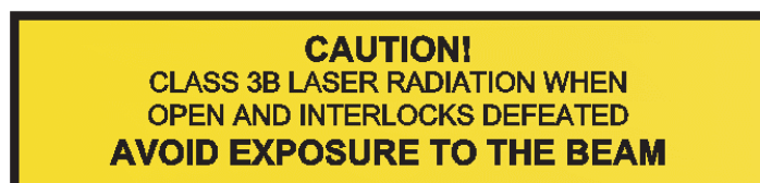
Fig. 1.2. Laser warning label.
