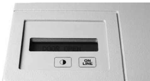
Fig. 4.1. PharosFX LCD and control panel.
