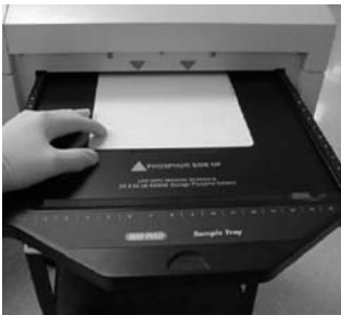
Fig. 4.13. Steps for inserting a phosphor screen into the scanner.
